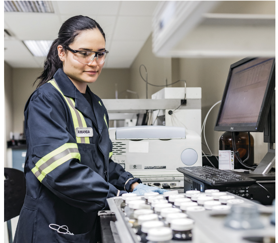
Toromont's laboratory services analyze machine oil for harmful contaminants that degrade performance and damage wear parts.
